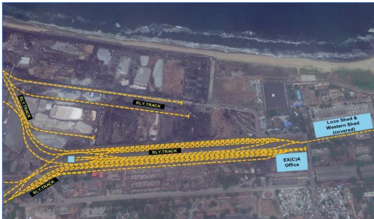
Figure 8-12: Railway Network at the Marshalling Yard
